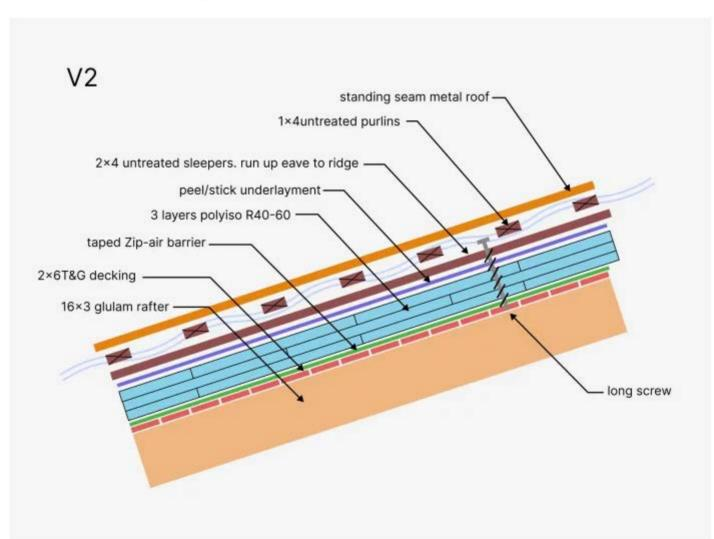
The revised assembly includes ventilating the low-slope roof to keep the sheathing cold in high-snow country.
